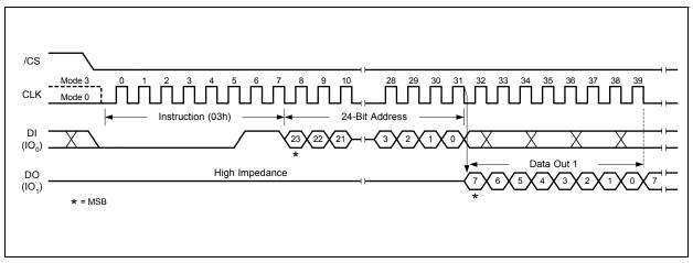
Figure 9. Read Data Instruction Sequence Diagram
