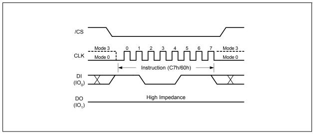
Figure 24. Chip Erase Instruction Sequence Diagram
