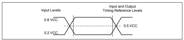
Figure 39. AC Measurement I/O Waveform
