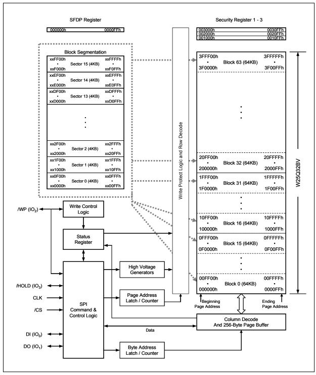
Figure 2. W25Q32BV Serial Flash Memory Block Diagram
