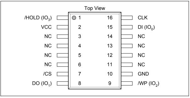
Figure 1d. W25Q32BV Pin Assignments, 16-pin SOIC 300-mil (Package Code SF)
