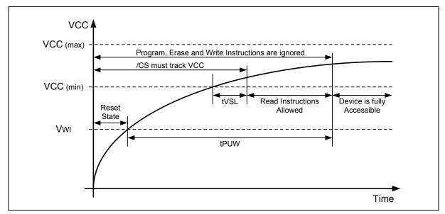
Figure 38. Power-up Timing and Voltage Levels
