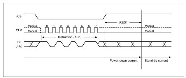
Figure 28a. Release Power-down Instruction Sequence
