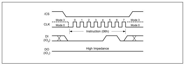
Figure 4. Write Enable Instruction Sequence Diagram
