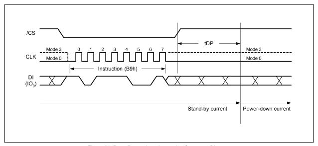
Figure 27. Deep Power-down Instruction Sequence Diagram
