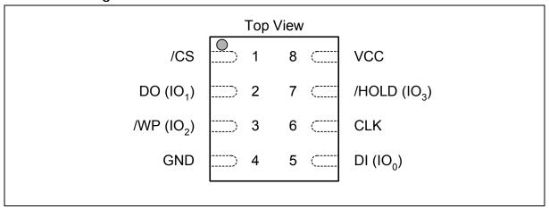
Figure 1b. W25Q32BV Pad Assignments, 8-pad WSON 6x5-mm / 8x6-mm (Package Code ZP, ZE)
