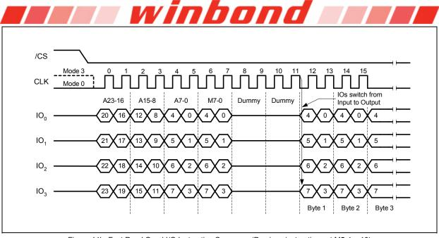
Figure 14b. Fast Read Quad I/O Instruction Sequence (Previous instruction set M5-4 = 10)
