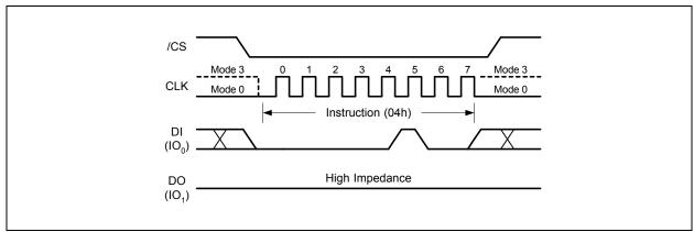
Figure 6. Write Disable Instruction Sequence Diagram
