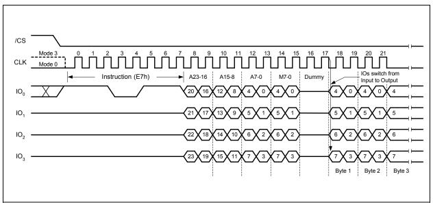
Figure 15a. Word Read Quad I/O Instruction Sequence (Initial instruction or previous M5-4  $\neq$  10)
